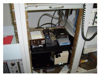
Here's a better look at the middle bay. The rig on the left is for local forwarding on 1.25 M, 10 watts output. The middle rig is the 70 cm 9600 baud user port, 4 watts output. And the one on the right is the 2 M 1200 baud user port, 10 watts output.
